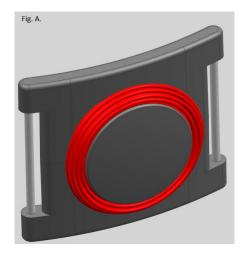
This module is alternately installed to a module of similar design, which allows the units to interlock as they are assembled about the circumference of the shaft. See figure B.
