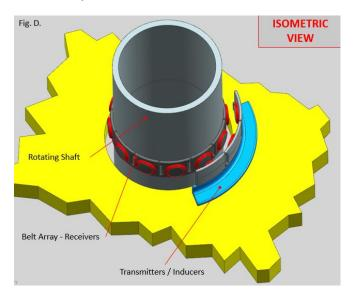
The Transmitter array would be energized by an external power supply and switchable at the base. It is composed of lightweight materials except for the base, itself.
